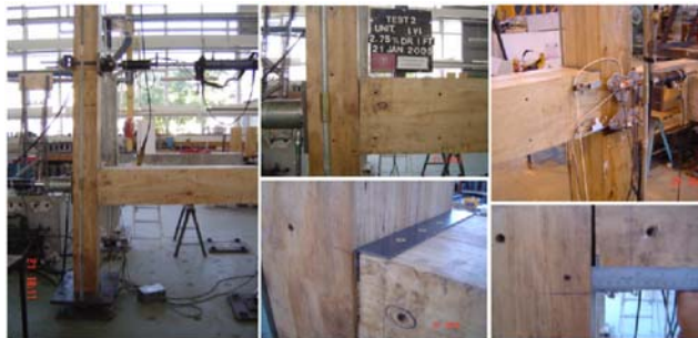
Figure 8. Unbonded post-tensioned solution: performance of the specimen ( 0.6 f_{py} ) at drift level of 2.75%.
