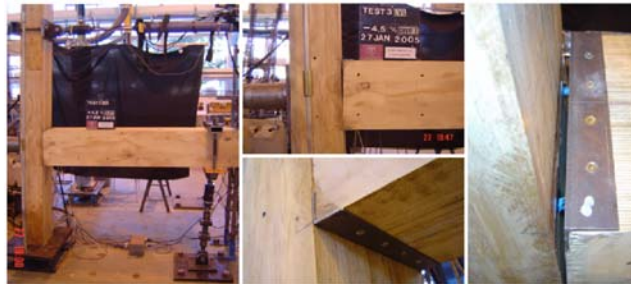
Figure 10. Hybrid solution: performance of the specimen at 4.5% drift.
