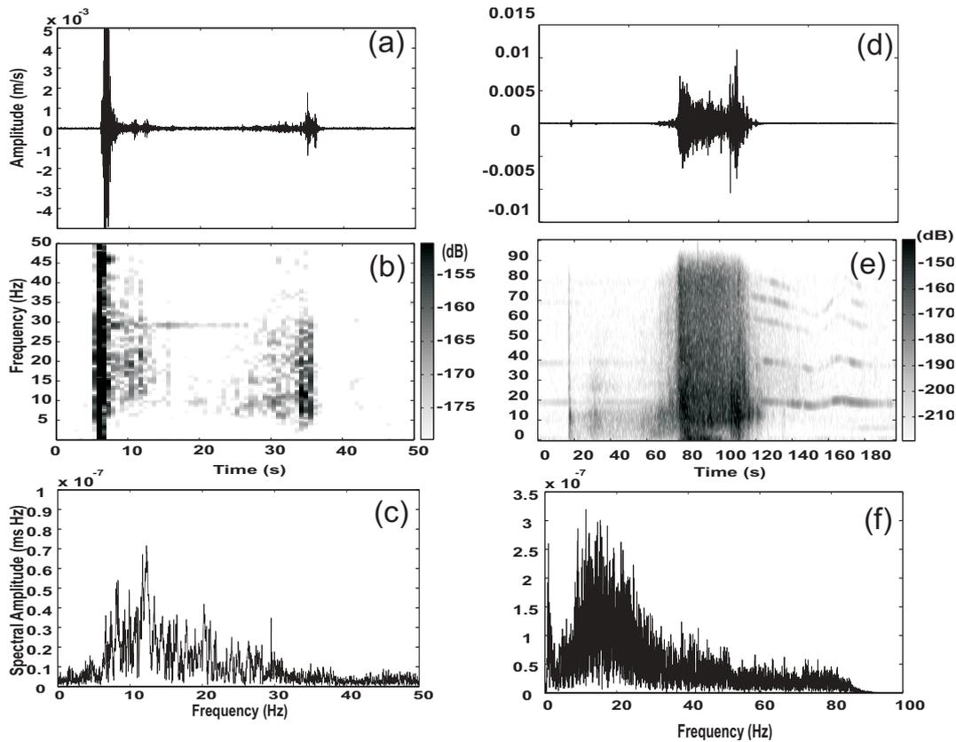
**Fig. 3.** Núría and Ryggfjonn avalanche signals. Top: seismograms; Middle: spectrograms (RS); Bottom: full spectra (TS). (a) E-W component seismogram (100 sps) of the Núría (Spain) artificially released wet snow avalanche on 1 February 1996. (b) N-S component seismogram (200 sps) of the Ryggfjonn site (Norway) artificially released dry-mixed snow avalanche on the 28 February 2004. Running spectra with a 128-sample window and 50% overlap.
