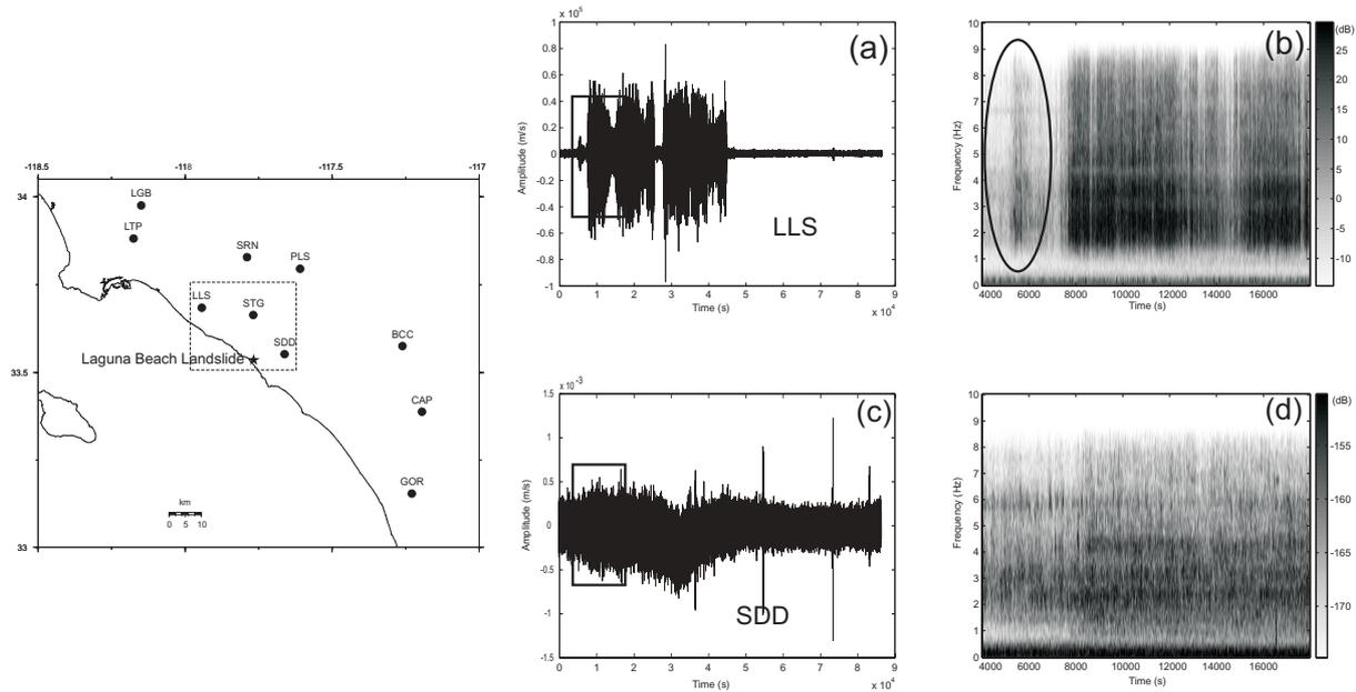
**Fig. 5.** Left: Map showing the Laguna Beach landslide (Star) and 10 closest seismic stations of Caltech/USGS Regional seismic network (CI). Centre: E-W component seismograms (20 sps) recorded at stations (a) LLS (23 km from landslide); (c) SDD (9 km from landslide); (b) and (d) spectrograms (RS) of (a) and (c) respectively with a 128-sample window and 50% overlap.
