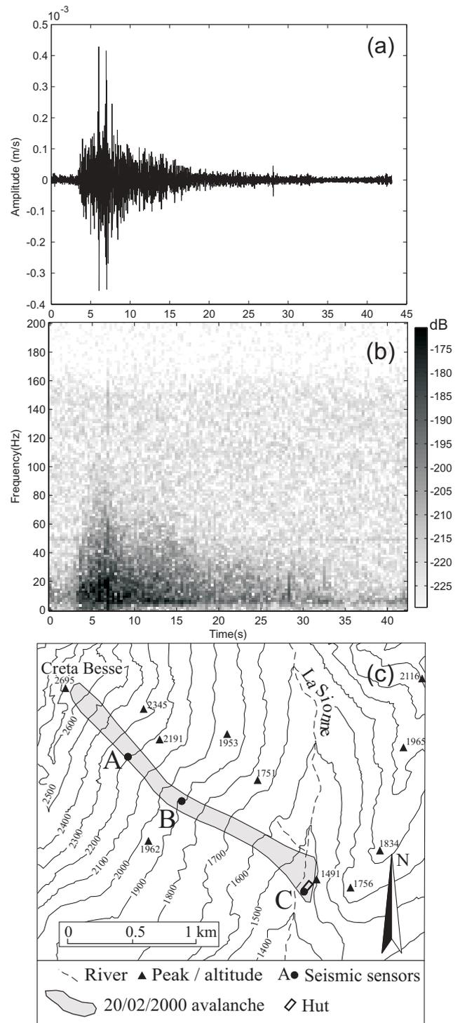
**Fig. 4.** (a) E-W component seismogram (400 sps) of La Sionne (Switzerland) artificially released dry/mixed avalanche of 20 February 2000 09:40 UTC, recorded at station A. (b) Running spectra with a 128-sample window and 50% overlap. (c) Cartography of the avalanche; A, B, C locations of the seismic sensors.
