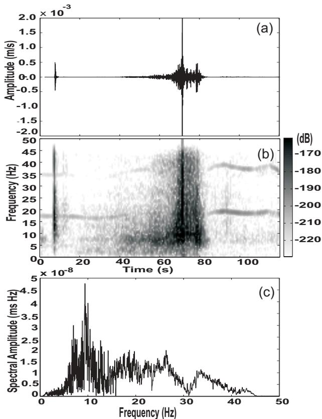
**Fig. 1.** (a) E-W component seismogram (100 sps) of La Sionne (Switzerland) artificially released dry/mixed avalanche on 20 February 2000, 09:40 UTC recorded at station C (Fig. 4c). (b) Running spectra with a 128-sample window and 50% overlap. (c) Total spectrum of the avalanche signals (excluding the explosion).
