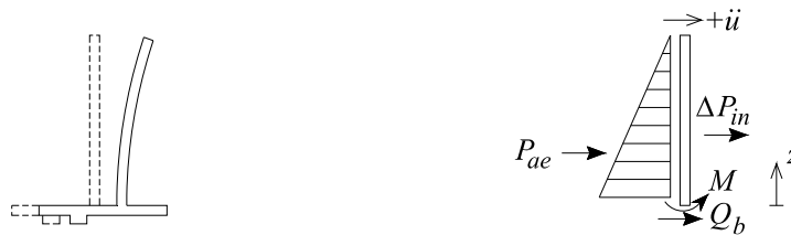
Figure 3.19 Vibration mode of cantilever wall and free body diagram; the sign convention for positive acceleration, loads and moments is indicated by the arrows.
