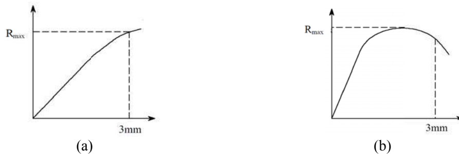
Figure 5.4 Failure limits for test (Source: ECCS TC7 TWG 7.10 Connections in Cold-formed Steel Structures, 2009)
