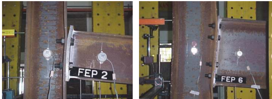
FIGURE 9: Failure mode at the end of the test.
