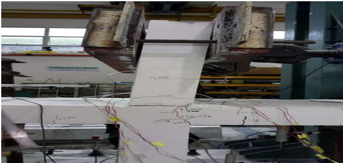
Fig.15. Cracks occurred at wall-slab joint
