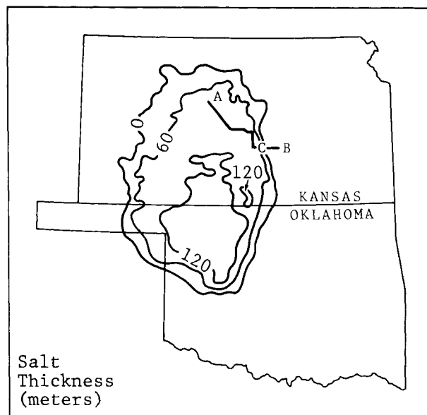
FIG. 1. Generalized extent and thickness of Hutchinson salt member of the Permian Wellington formation. Location of cross-section A-B is shown for Figure 2. The sinkholes discussed are located within a few kilometers of A. Modified from Walters (1977).
