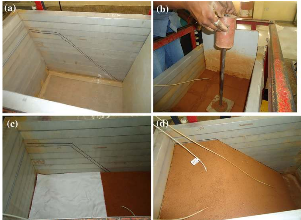
Fig. 5 Sequence of model slope construction: a marking slope geometry, b soil compaction in layers, c placing reinforcement between layers, d finished model slope
