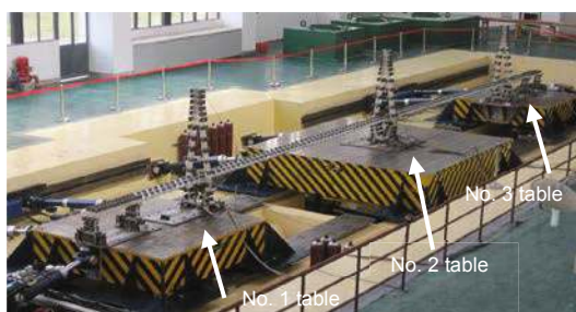
Fig. 2 Three-tower cable-stayed bridge model test
