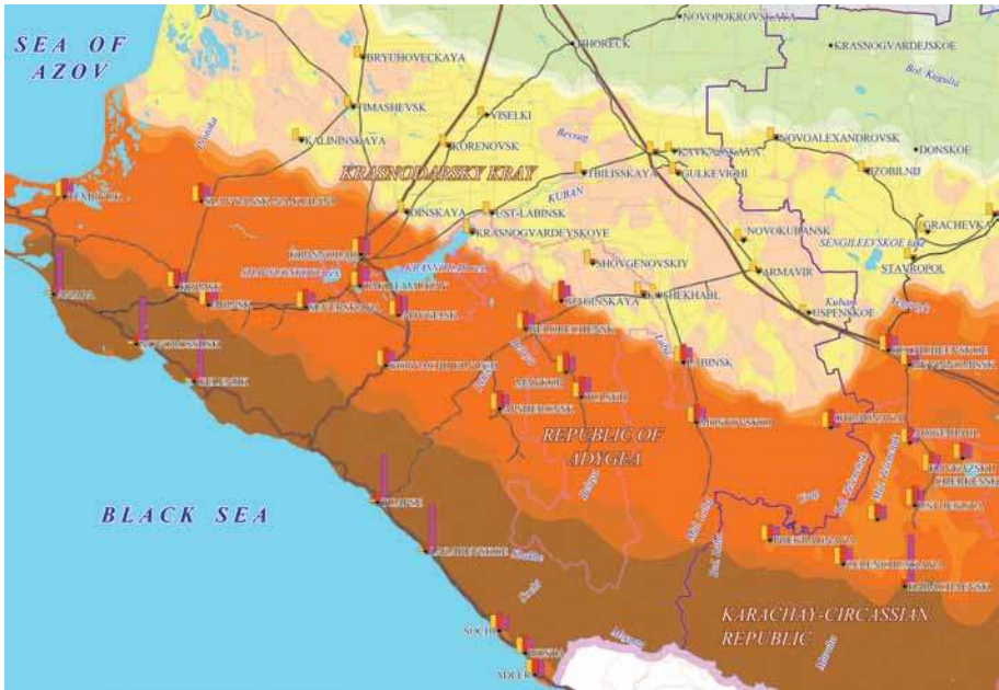
Fig. 14. Fragment of the physical vulnerability map for the Northern Caucasus Federal region of the Russian Federation and Krasnodar area: percent of buildings in settlements which may survive damage states d = 3, 4, 5 in the case of earthquakes according to the seismic hazard map OSR-97B:
