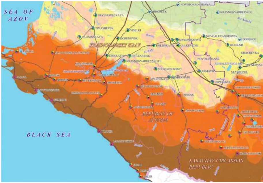
Fig. 13. Fragment of the physical vulnerability map for the Northern Caucasus Federal region of the Russian Federation and Krasnodar area: percent of buildings in settlements which may survive damage states d = 1, 2, 3, 4, 5 in the case of earthquakes according to the seismic hazard map OSR-97B:
