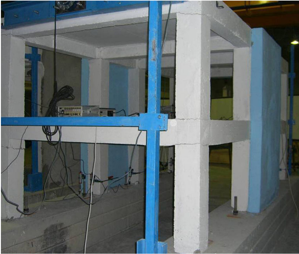
Figure 11. Damaged SM after the test.
