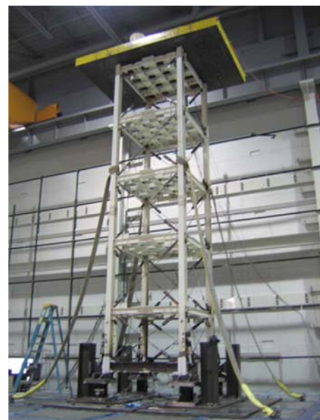
Fig. 2. Rocking steel truss pier specimen on shake table
