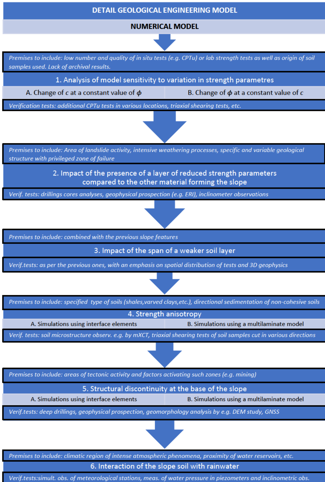
Figure 1: Flowchart of the factor-by-factor numerical analysis approach
