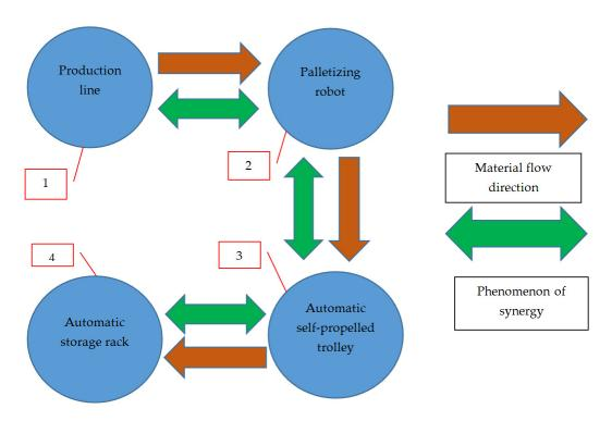
Figure 5. Material flow and synergy between machines.
