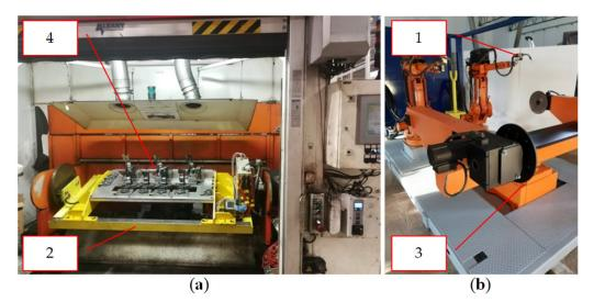
**Figure 2.** Welding cell: (**a**) view from the operator's side; (**b**) view from the robots' side (executive part of the cell).
