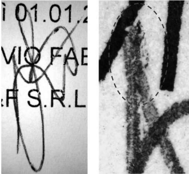
Figure 7. Questioned initials X. On the left is the scan of the signature, on the right a photograph of the same fragment taken with the digital microscope. Examination under the microscope revealed a thin stroke going outside the path of the main stroke and separating from it. At the point marked with the arrow the angle difficult to imitate was made in two attempts. Magnification showed presence of traces of ink distributed outside the path of the main stroke
