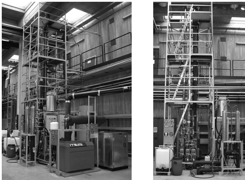
Figure 5. Gas-fired mini plant for post combustion carbon dioxide capture at ITT, University of Stuttgart. Left: overall view with gas burner. Right: absorber and desorber
