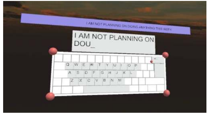
Figure 3. This figure shows the virtual environment including stimulus (purple), text input field, and the virtual keyboard.
