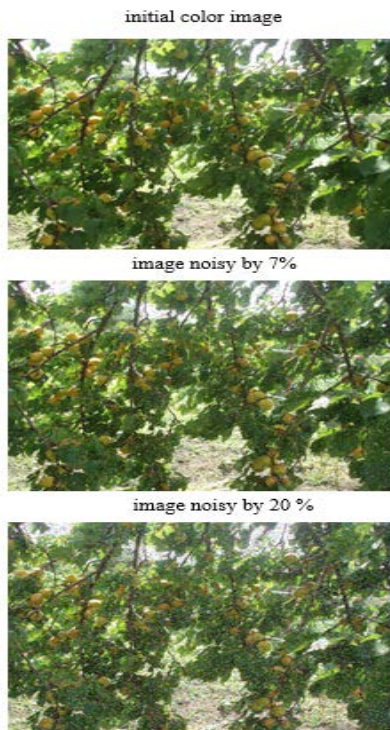
Fig. 8 An example of the introduction of noise such as "salt" and "pepper".
