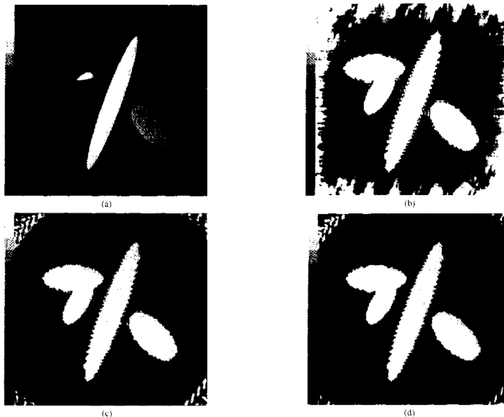
Fig. 6. Reconstructed images of a numerical phantom consisting of four ellipses, showing the effect that the convolution function has on the resulting image. Image (a) was reconstructed using a width three Kaiser-Bessel window ( \beta = 4.2054 ), without subsampling. Image (b) is the same as image (a), but scaled from 0 to 5% to show the error in the reconstruction. Image (c) was reconstructed using a width three, two-term cosine window [0.5068 + 0.4932 \cos(\pi u/1.5)] on a subsampled grid, and is scaled the same as image (b). Image (d) was reconstructed using a width three, Kaiser-Bessel window ( \beta = 13.9068 ) on a subsampled grid, and is also scaled the same as image (b).
