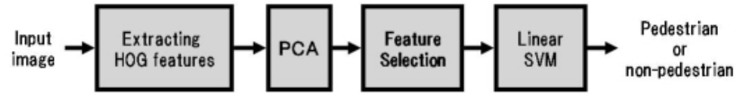
Fig. 1. The overview of our pedestrian detection algorithm. The HOG features are extracted from all locations in an image grid. Then PCA is applied to the extracted HOG features to reduce the dimensionality (PCA-HOG features). A proper subset of these PCA-HOG features are selected to improve the generalization. The selected PCA-HOG features are used as an input vector of the linear SVM.
