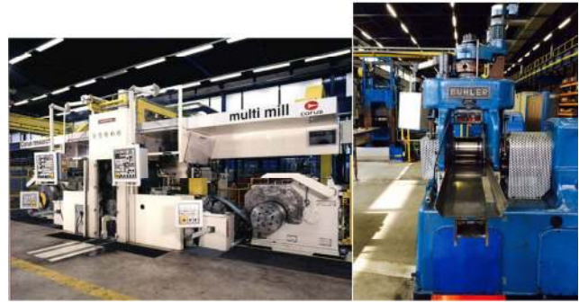
Fig. 17 Overview of the pilot rolling mills at Tata Steel, used for rolling trials in Steeltac: (left) 4-high Multimill, and (right) 2-high “Bühler” mill, used for the STEELTAC project [69].
