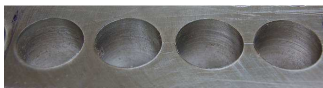
Figure 1. The observed burrs at the exit of holes during drilling experimentation for 16 mm drill diameter.
