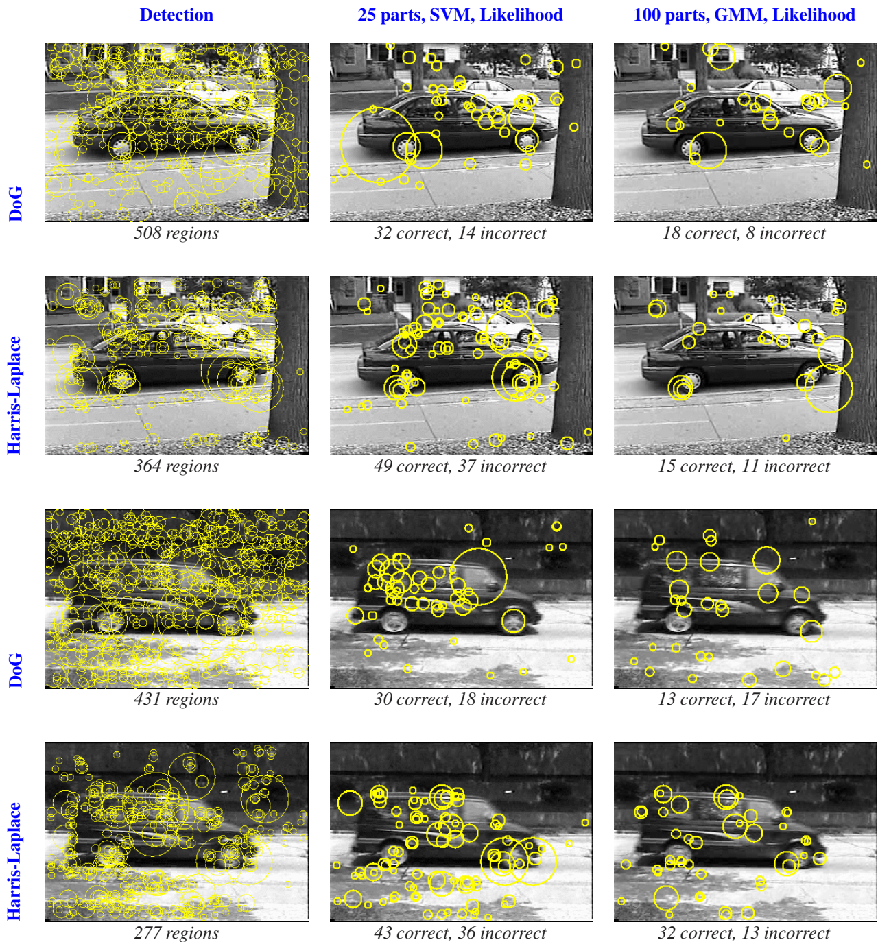
Figure 7. Results for two test images. The left column shows the interest regions detected with DoG and Harris-Laplace. The middle column displays the descriptors classified by the 25 best SVM classifiers selected with the likelihood ratio. The right column shows the results for the 100 best GMM classifiers selected with likelihood ratio.
