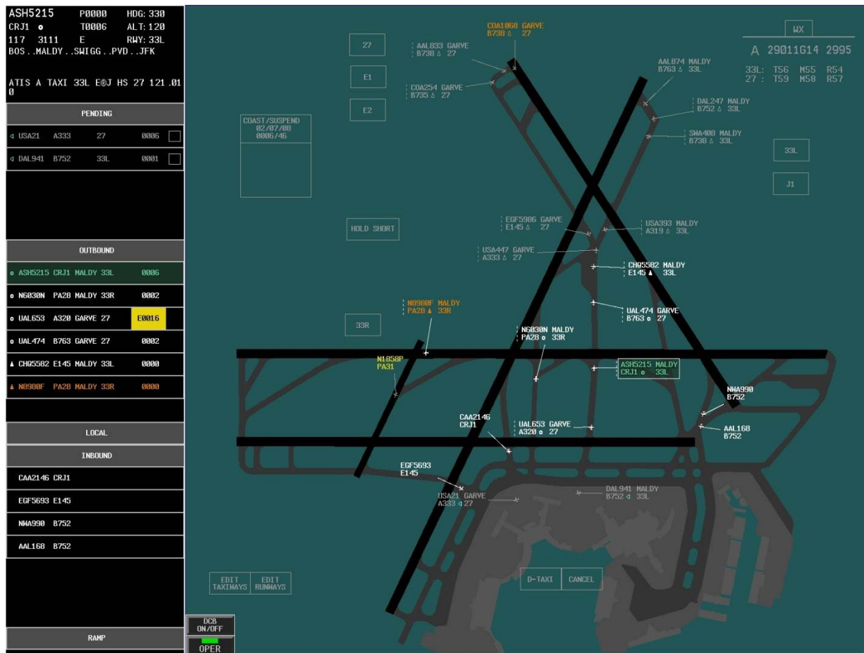
Figure 16: Example future electronic flight strip bay (left) and airport surface display (right) (photo courtesy of Todd Truitt, FAA Technical Center)
