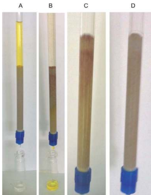
Fig. 10 (A) Decoloration of a \text{Cr}_2\text{O}_7^{2-} solution (initial concentration = 1075 ppm, pH \sim 3) with an ion-exchange column of MOR-1-A/sand (0.05 : 5 g). (B) Regeneration of the \text{Cr}_2\text{O}_7^{2-} -loaded column by washing it with 4 M HCl solution. (C) Column with the stationary phase saturated with \text{Cr}_2\text{O}_7^{2-} . (D) Column after the regeneration process.
