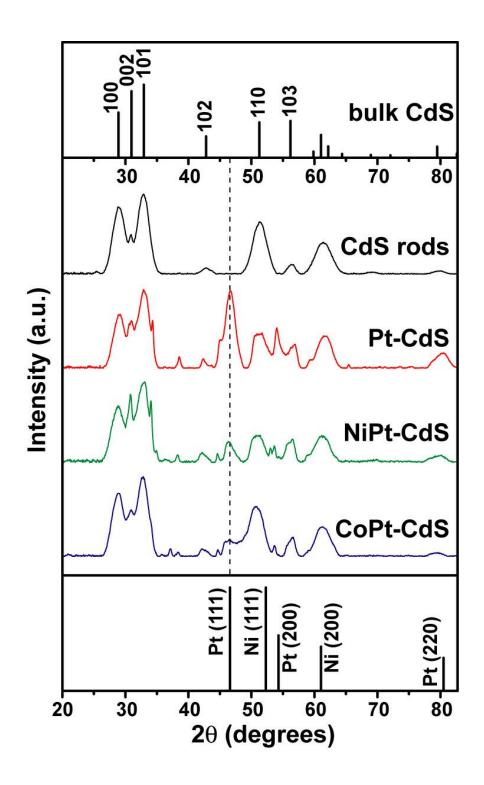
*Figure S2.* Complete set of XRD spectra for pure CdS nanorods, and heterostructures of CdS-Pt, CdS-PtNi, and CdS-PtCo, with bulk diffraction values for pure CdS, Pt, and Ni.
