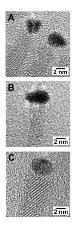
Figure S1. Enlarged HRTEM images of (A) Pt-CdS, (B) PtNi-CdS, and (C) PtCo-CdS heterostructures.
