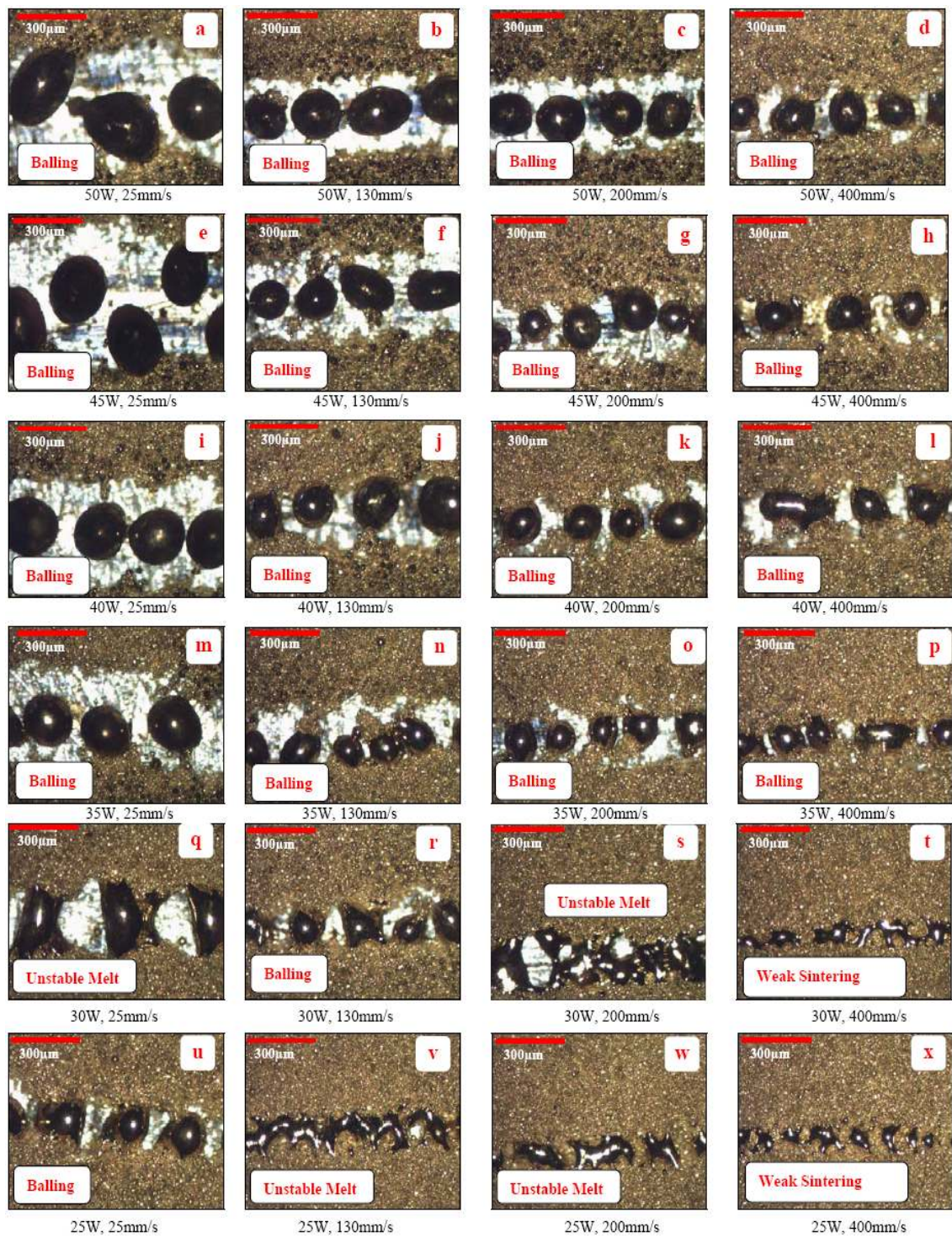
Figure 8-4: (a-x) Balling, unstable melt and weak sintering at different laser power and scan speeds (all images were taken at same magnification)
