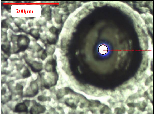
Figure 7-6: Spot size measurement (35µm) for YLM-50 laser on black burn paper
