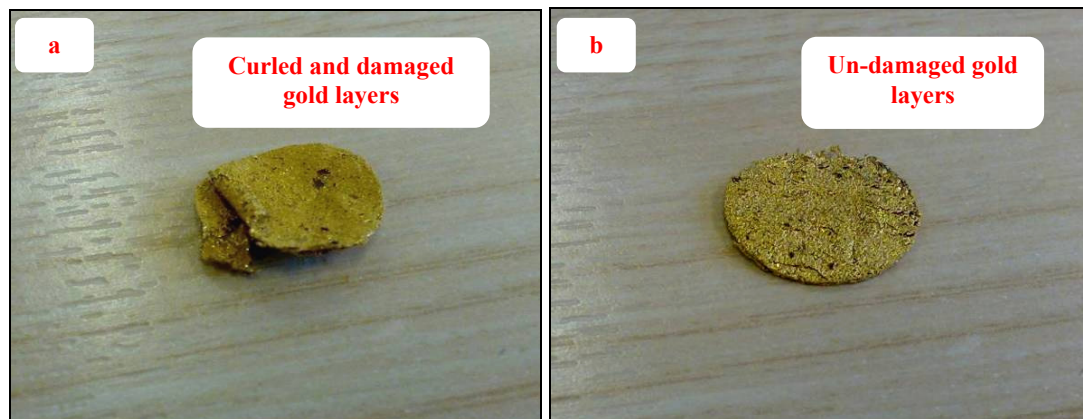
Figure 9-6: Multiple layer gold discs (a) bed temperature 28°C (room temperature) (b) bed temperature 100°C
