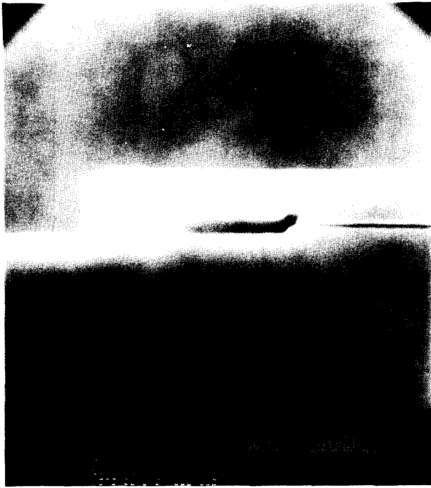
FIG. 3. SEM picture showing a magnified view of the etched channel of the wafer placed at the hot end of an ampoule after heating. The dark thin region on the right is the InGaAsP layer. The region to the left of the InGaAsP layer is the etched undercut channel (see Fig. 1), which is seen to be etched to about four times its original thickness (scale = 1\ \mu\text{m} ).
