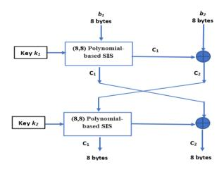
Figure 7. The block diagram of the proposed F function
