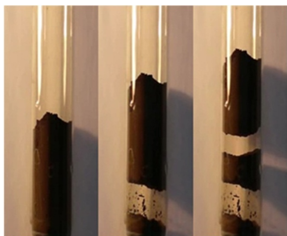
Figure 2 Slugging of iron-chromium catalyst.
