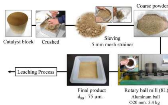
Fig. 2 Spent automotive catalyst pre-leaching treatment
