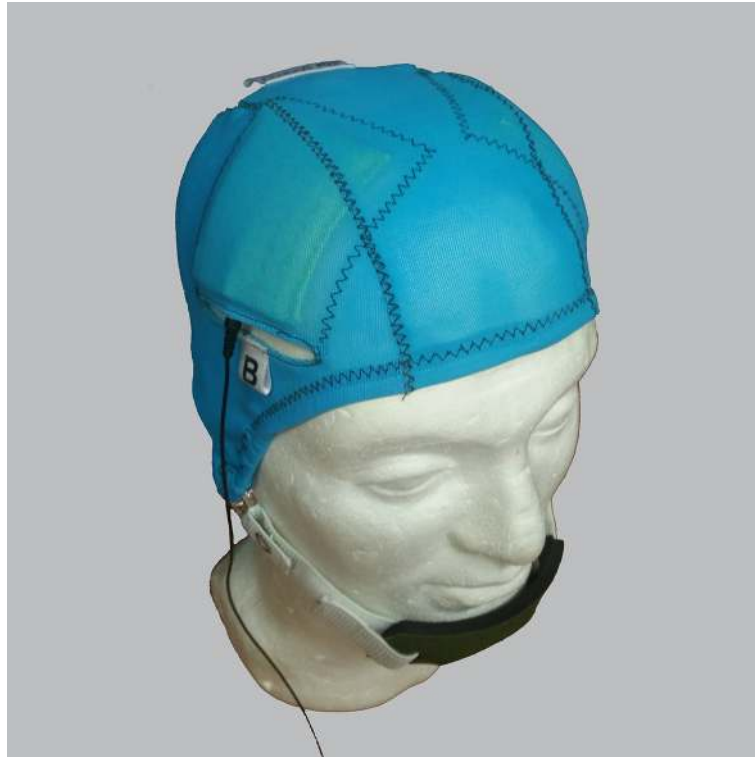
Fig 1. Custom-made tDCS electrode cap with sewn-on electrode positioning guides. Figure shows the cap for the bifrontal electrode montage. A different cap was used for the LTA montage.
