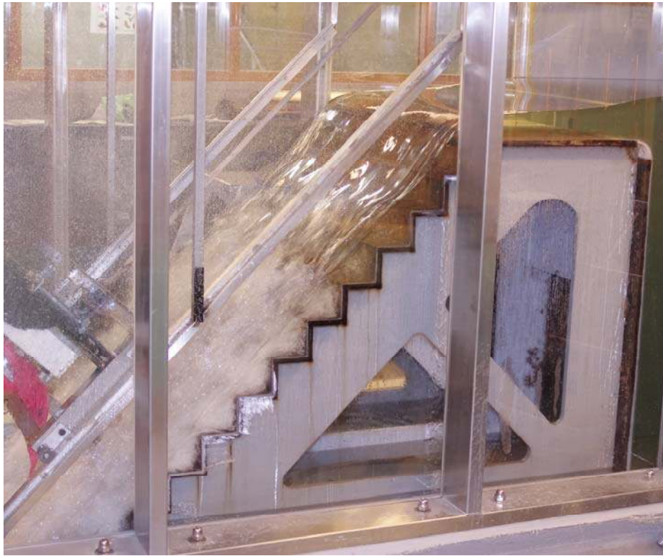
Fig. 5 - Free-surface aeration in a large-size stepped spillway model ( \theta = 45^\circ , h = 0.10 m, W = 0.985 m)
