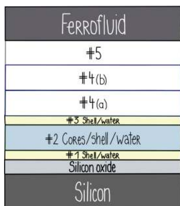
Figure 6. Sketch of the stack assumed for the fits of the neutron reflectivity data.
