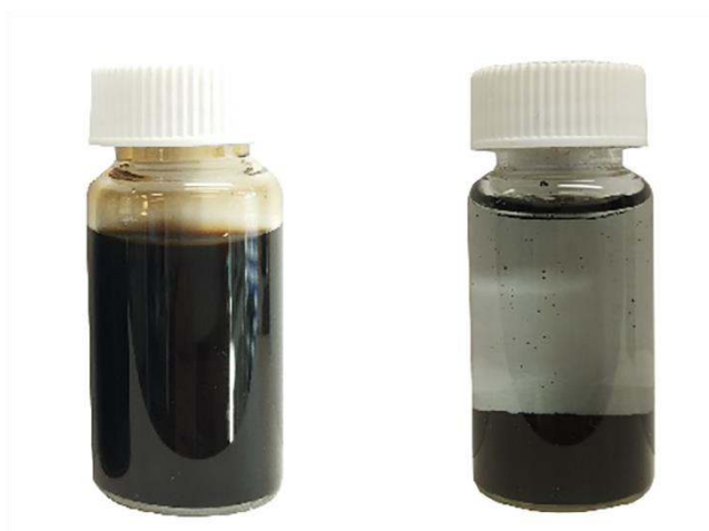
Figure S1. LCGO dispersion (left) and MoS 2 dispersion (right) after heating at 70 °C overnight.
