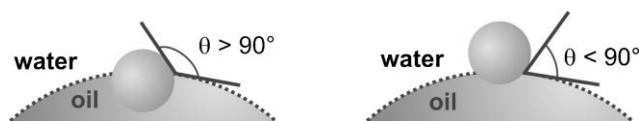
Fig. 2 Changes in wettability of solid particles at the oil/water interface at contact angles >90^\circ and <90^\circ .
