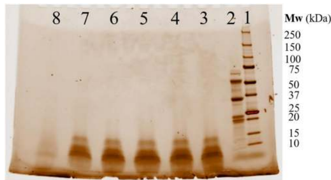
Figure 11. Representative SDS-PAGE results of protein, fibril and NP-fibril samples with different concentration of NPs. (lane 1), protein ladder; (lane 2), protein control; (lane 3) fibril control. (Lane 4–8) are results for NP-fibril samples. (lane 4), 0.0003 wt. % NP; (lane 5), 0.0015 wt. % NP; (lane 6), 0.003 wt. % NP; (lane 7), 0.03 wt. % NP; (lane 8), 0.3 wt. % NP.
