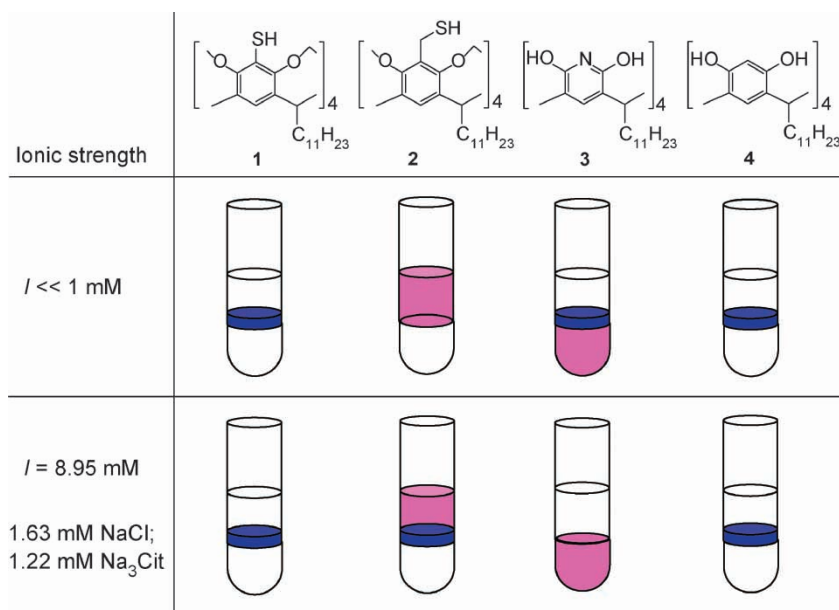
FIGURE 3 Illustrations of nanoparticle extractions by resorcinarenes 1–4, in the absence and presence of aqueous electrolyte. Self-assembled nanoparticle films at the aqueous interface appeared dark blue.
