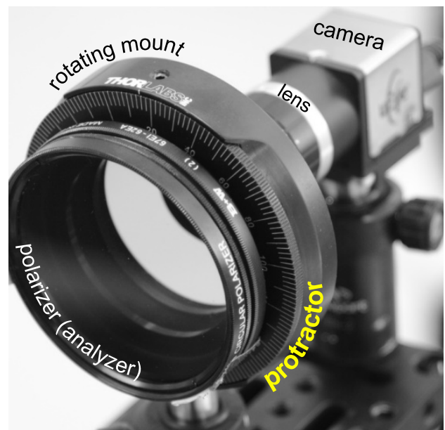
Figure 1. Polarimetric imaging has typically required a polarizing filter (analyzer) set to known angles. Commonly, the filter rotates using a controlled closed-loop motor, or manually with a fine protractor. This work seeks to dismiss the fine protractor or control, and still enable polarimetric imaging. Thus, the simplicity of uncontrolled amateur photography can be tamed for scientific measurements.
