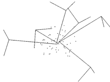
Figure 4. Example of sequence used for simulations (the views are represented by the optical axis and the image axes of the camera in the different positions).
