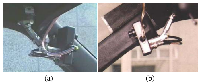
Fig. 2 THE CAMERAS INSTALLED INTO THE DRIVING CABIN: (a) INTERNAL VIEW AND (b) INTERNAL VIEW AFTER A SHADOWING DEVICE HAS BEEN PLACED ON THE WINDSHIELD TO PREVENT FROM DIRECT SUNLIGHT OVERHEATING AND INTERFERING WITH THE CAMERA.
