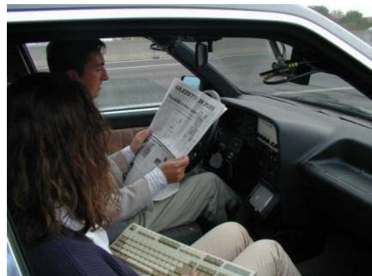
Fig. 1 ARGO DRIVING IN AUTOMATIC MODE; THE ON-BOARD INSTRUMENTATION IS VISIBLE.
