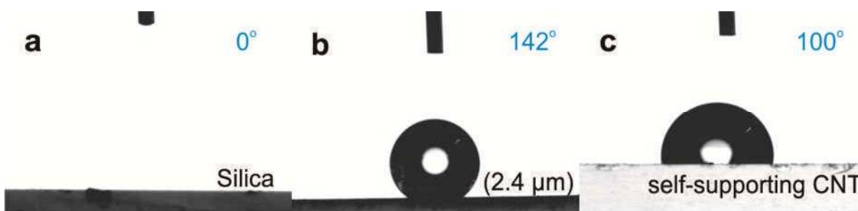
33 Figure 4. Water contact angles of (a) macroporous silica substrate, (b) CNT-silica bi-layered 34 material with CNT layer thickness of 2.4 \mu\text{m} and (c) self-supporting CNT membrane. 35 36
