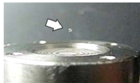
FIG. 7. (Color online) Photograph showing the ejection of a glycerin droplet at a liquid depth of 2.5 mm.
