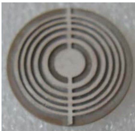
FIG. 3. (Color online) Photograph of a milled FZP with six annular electrodes.
