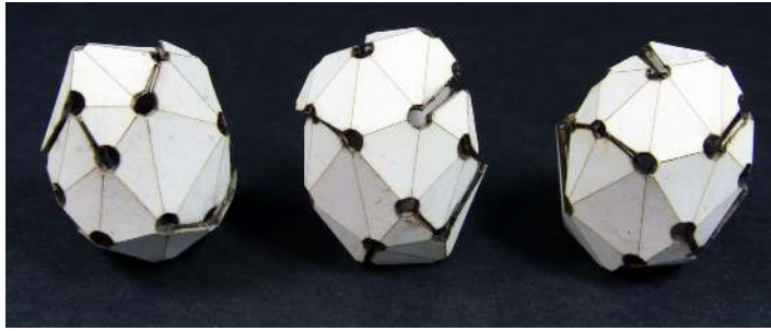
Figure 7. Repeatability of folding. Several challenges limited the repeatable self-folding of complex structures, including the number of serial folds, and the differential effect of gravity on the faces of the object depending on their size and position in the structure.
