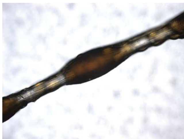
Figure 32. An image of a compartmented alginate fiber encapsulating rejuvenator captured by optical microscope. Plane polarized light imaging. Field of view is \approx 3 mm. Reproduced with permission. [19] Copyright 2016, IOP Publishing Ltd.
