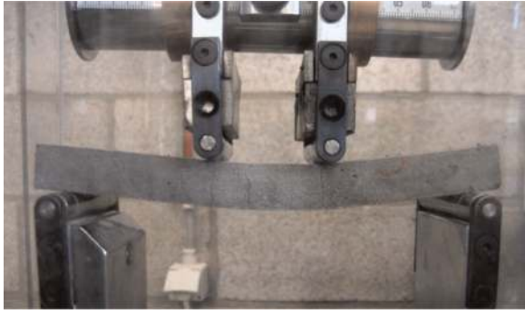
Figure 5. Four-point-bending test on a specimen containing 2 vol.% of PVA fibres showing a vertical displacement of 7 mm. The total height of the specimen is 15 mm. PVA: polyvinyl alcohol.
