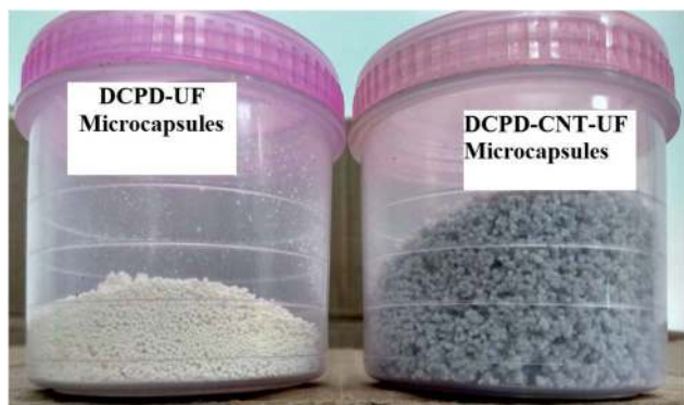
Fig. 1 DCPD-UF and DCPD-CNT-UF microcapsules synthesized in this study.
