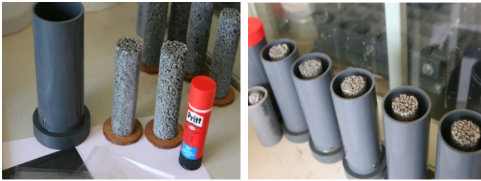
Fig. 9 Casting preparation where porous concrete cylinder was placed in the center of the mould and normal strength self compacting concrete was poured around.
