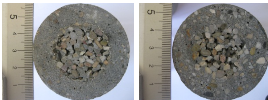
Fig. 11 a) Left; more regular circle of porous core due to PVA film cover, and b) Right: irregular boundary due to penetration of cement paste into uncovered porous core.
