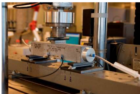
Fig. 17 Three points bending test for crack formation showing injection connector and LVDT.
