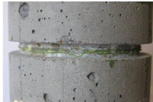
Fig. 14 Crack formation of concrete cylinder in the notch.
