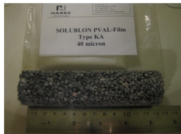
Fig. 8 Porous concrete cylinder that would be used as porous core in PNC samples.
