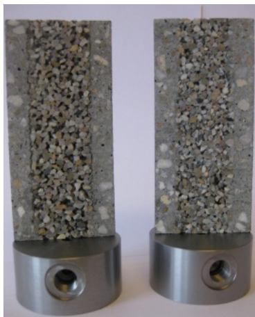
Fig. 10 Bone-like concrete; a new hierarchical material is made in which sponge-like core is surrounded by solid concrete.
