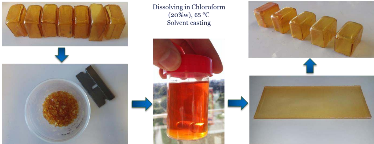
Fig. S 17: Diels-Alder polymer waste of the manufacturing process of the prototypes can be recycled. This was proven by recycling the DPBM-FGE-J4000 cuboid cells. The cells were cut into small pieces and these were subsequently swelled and dissolved in chloroform (20 w%). To increase accelerate the dissolving, the mixture was heated up to 65 °C. A sheet (0.75 mm) was solvent-cast and from this sheet cells were constructed.
