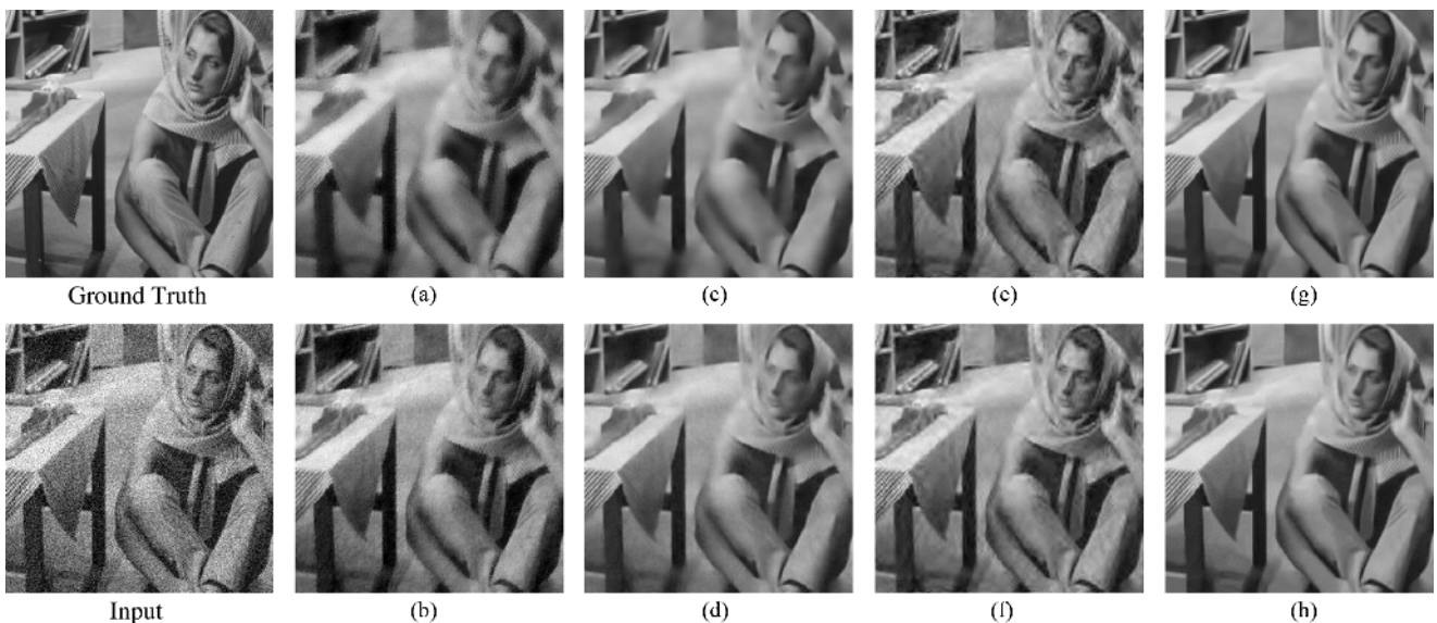
Fig. 12. Example image denoising results. Note that the input image is the noisy version of ground truth image (with Gaussian noise). Denoising outputs are produced by the methods of (a) Bilateral [12], (b) ours with Bilateral, (c) K-SVD [7], (d) ours with K-SVD, (e) SURE-LET [26], (f) ours with SURE-LET, (g) BM3D [13], and (h) ours with BM3D.
